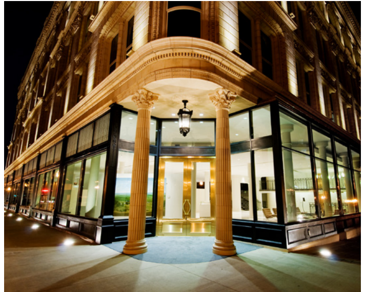
Effective building lighting combines internal storefront lighting and external illumination of architectural features.
